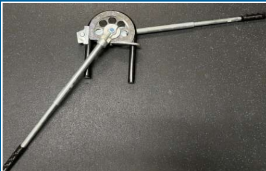
Imperial 1" lever tube bender
